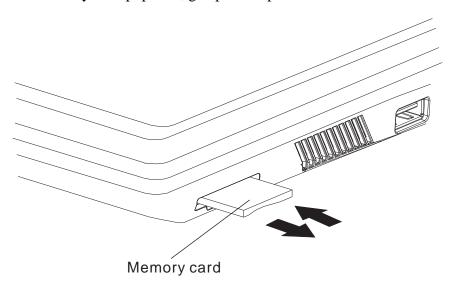
Figure 4-2 Removing the memory card
